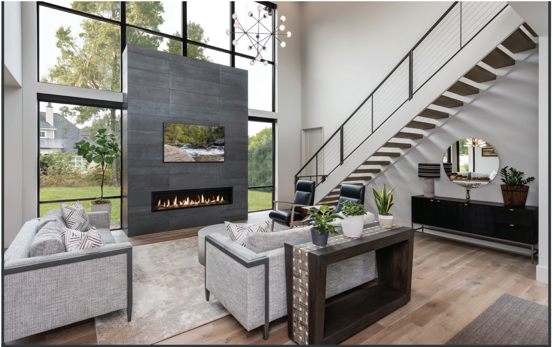
The custom fireplace is direct vent gas with an exterior brick wall and an interior composed of long-format linear tiles. A frame television embedded over the flames can display art or any form of network entertainment.
